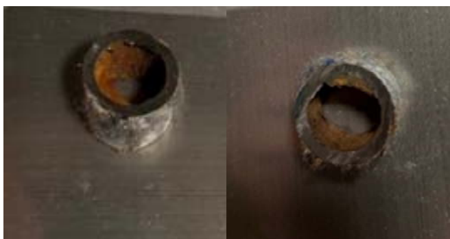
Figure3: Example of preparation of a test piece of the pipe
